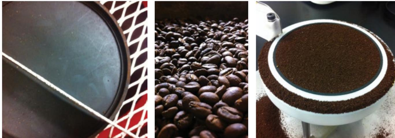
**LEFT** Flat-edged leveling tool on an Agtron sample dish. **CENTER** Thorough cooling before evaluating color is critical for quality measurements and product quality. **RIGHT** A prototype of a leveling device designed for sample preparation, pictured with an Agtron sample dish.
